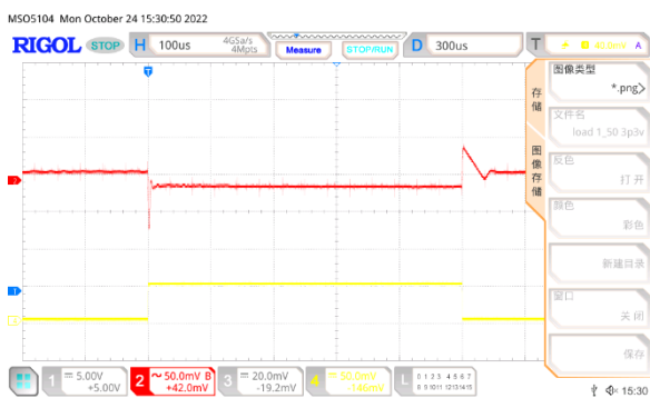
Load transient V_{OUT}=3.3V , I_{OUT}=1mA-50mA
