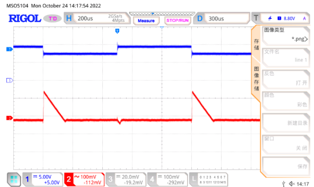
Line transient V_{OUT}=5.0V , I_{OUT}=1mA
