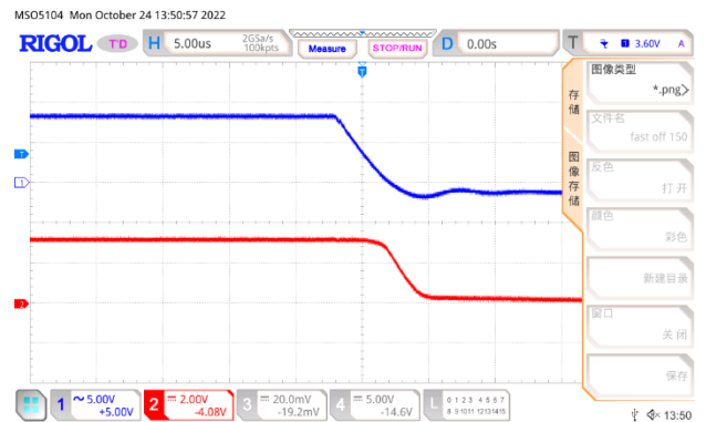
V_{IN} fast off 150mA, V_{OUT}=3.3V
