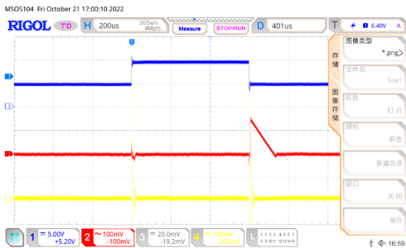
Line transient V_{OUT}=3.3V , I_{OUT}=1mA
