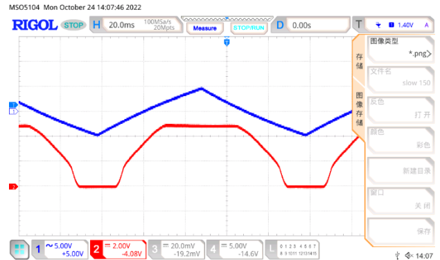
V_{IN} slow on/off 150mA, V_{OUT}=5.0V
