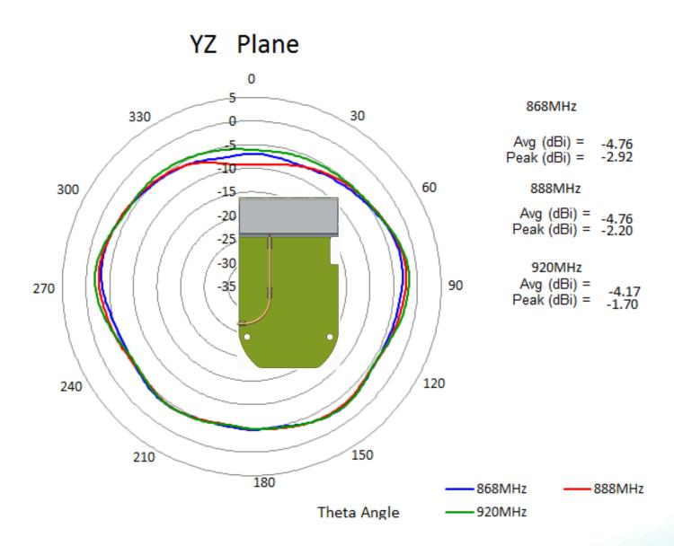
Test PCB size: 67.8mm\*39.6mm
