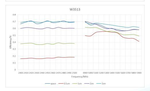
When the distance is 0.5-2cm, the metal mainly affect the performance of low frequency band(2.4G-2.5G). When the distance is above 2cm, the metal will have a little influence in two band.
