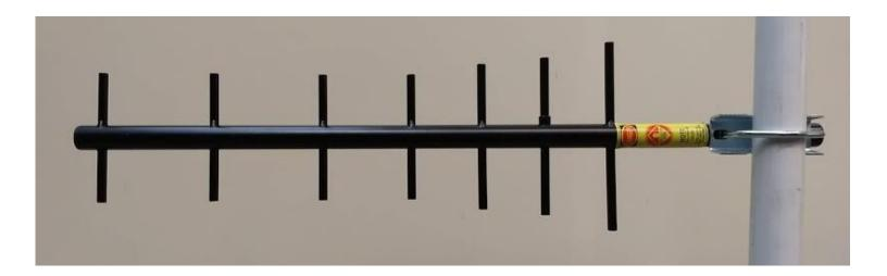
Antenna mounted vertically on post with insulator on driven element facing up
