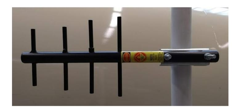
Antenna mounted vertically on post with insulator on driven element facing up
