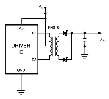
For a fixed 50% duty cycle mode of operation, the output voltage is simply determined by the input voltage and turns ratio. So, with the available turns ratios, a variety of output voltages can be selected.
