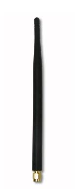
Pulse is proud to introduce a ruggedized line of ISM antennas for North American and European applications. These IP-65 rated antennas covering 868 to 928 MHz are suitable for either European or North American operations. The antennas are both supplied in a slim 179 mm (7 inch) package. The W5017 has an SMA-Male connector while the W5012 has SMA RP-Male.
