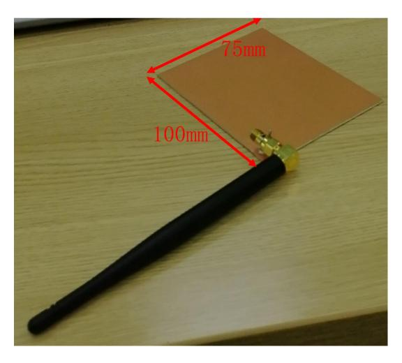
Test with a 100mm\*75mm ground plane in free space.
