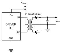
For a fixed 50% duty cycle mode of operation, the output voltage is simply determined by the input voltage and turns ratio. So, with the available turns ratios, a variety of output voltages can be selected.
