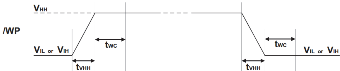
Figure 66. ACC Program Acceleration Timing and Voltage Levels
