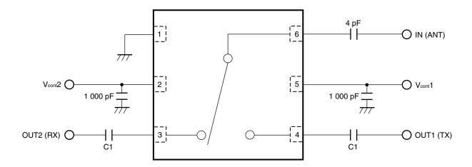
Remark C1: 2.4 to 2.5 GHz and 4.9 to 6.0 GHz 4 pF 8.0 GHz 2 pF 0.5 to 2.5 GHz 100 pF
