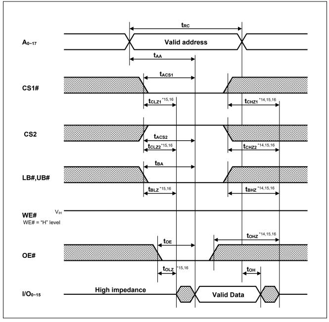
Note 14. t<sub>CHZ1</sub>, t<sub>CHZ2</sub>, t<sub>BHZ</sub> and t<sub>OHZ</sub> are defined as the time when the I/O pins enter a high-impedance state and are not referred to the I/O levels.
