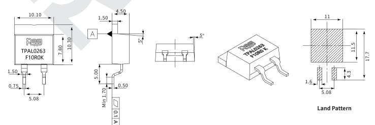
Note: The above dimensional tolerance is  $\pm$  0.3 mm.
