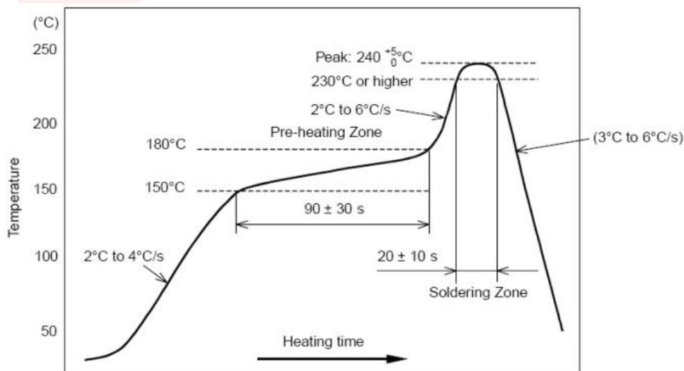
部件的焊接耐热性温度曲线(焊接点)
