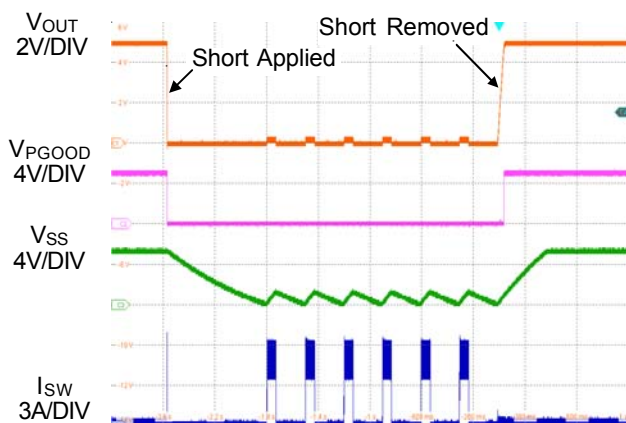
Figure 3. Short Circuit Protection and Recovery
