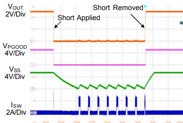
Figure 3. Short Circuit Protection and Recovery
