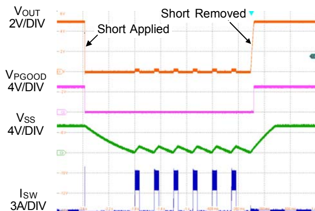
Figure 3. Short Circuit Protection and Recovery
