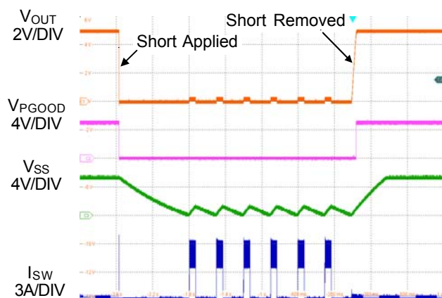
Figure 3. Short-Circuit Protection and Recovery
