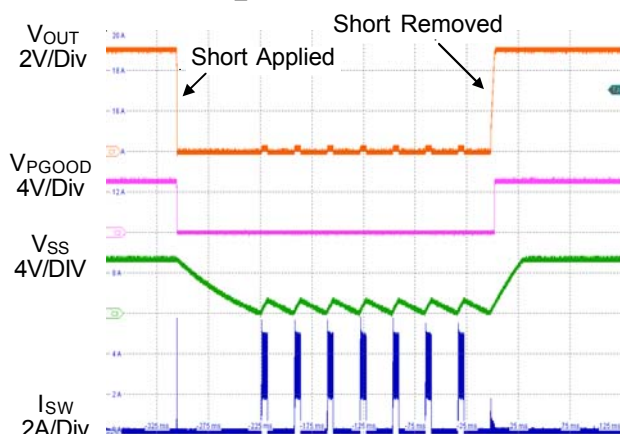
Figure 3. Short Circuit Protection and Recovery
