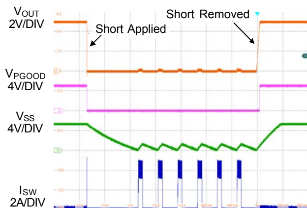
Figure 3. Short-Circuit Protection and Recovery
