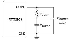
Figure 8. External Compensation Components
