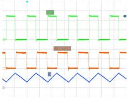
Figure 16. Synchronization Mode in CCM
