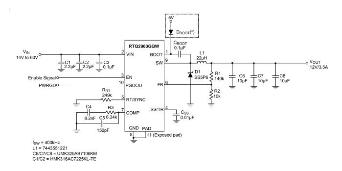
\*: While the input voltage is below 5.5V or duty ratio is higher than 65%, an external bootstrap diode must be added between an external 5V voltage supply and the BOOT pin to enhance the drive capability for the high-side MOSFET. Refer to the Application Information for more details on the external bootstrap diode design.
