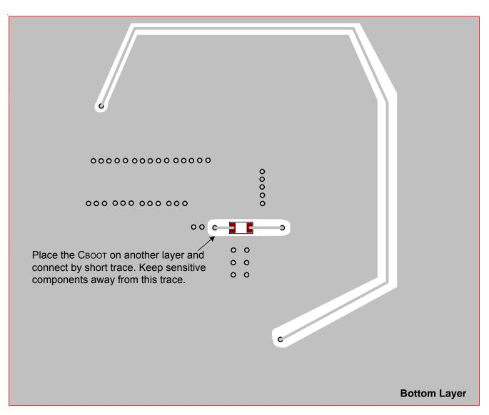
Figure 18. Layout Guide for RTQ2963GQW (Bottom Layer)
