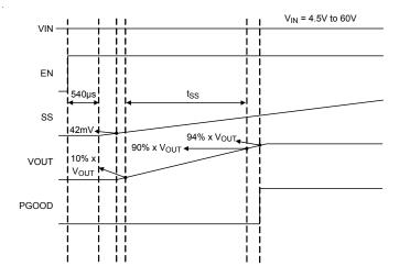
Figure 1 Start-Up Sequence for RTQ2963GQW
