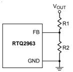
Figure 7. Output Voltage Setting
