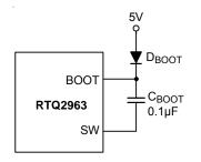
Figure 10. External Bootstrap Diode
