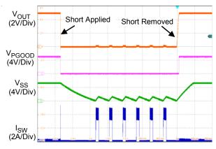
Figure 3. Short-Circuit Protection and Recovery
