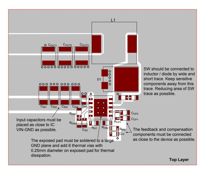
Figure 17. Layout Guide for RTQ2963GQW (Top Layer)
