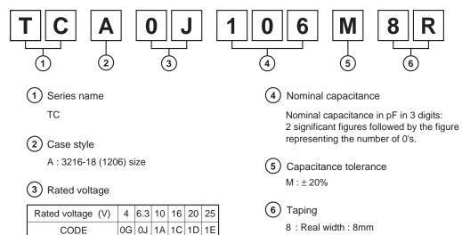
R : Positive electrode on the side opposite to sprocket hole
