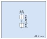
The recommended thickness of the screen mask for soldering is between 100 and 150 $\mu m$ . The hole size of the screen mask should be same as the recommended land pattern or smaller.
