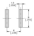
**Recommended Soldering Pad Layout**
