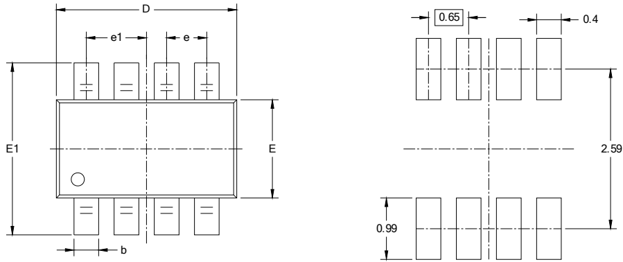
RECOMMENDED LAND PATTERN (Unit: mm)
