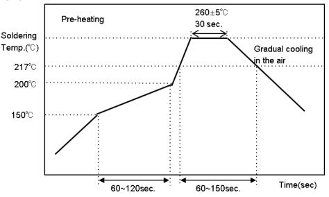
[Reflow Soldering Conditions]
