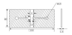
$\sim$  Thickness : T=1.6 mm (T= 0.8 mm for 02/03/05)
