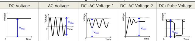
[Types of Voltage Applied to the Capacitor]
