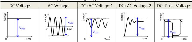
[Types of Voltage Applied to the Capacitor]
