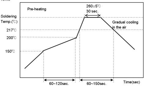
[Reflow Soldering Conditions]
