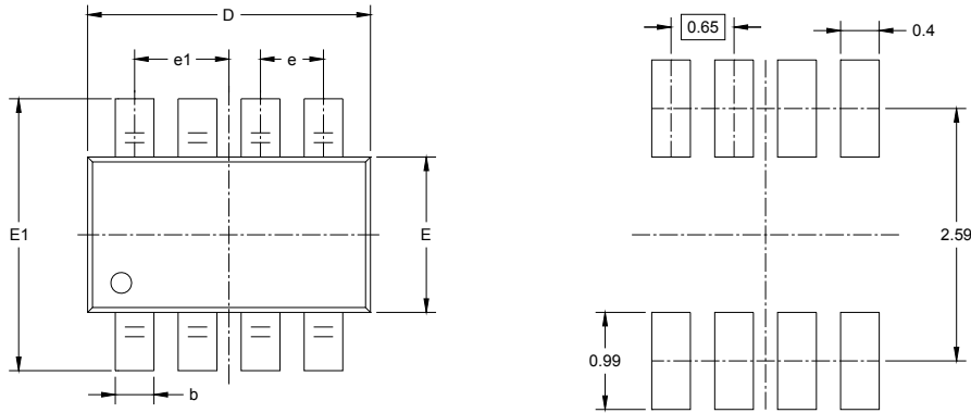
RECOMMENDED LAND PATTERN (Unit: mm)
