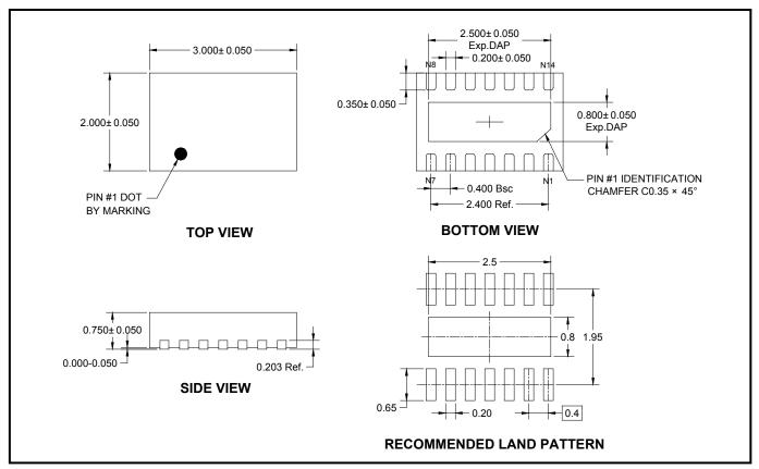
NOTE: All linear dimensions are in millimeters.
