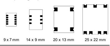
Industry's smallest 9.0 x 7.0 x 6.5H mm OCXO, plus 3 industry standard packages for drop-in replacement of quartz
