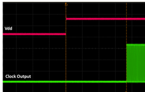
Figure 17. Startup Waveform vs. Vdd
