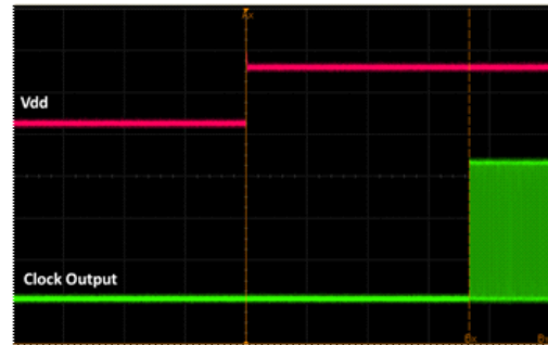
Figure 16. Startup Waveform vs. Vdd
