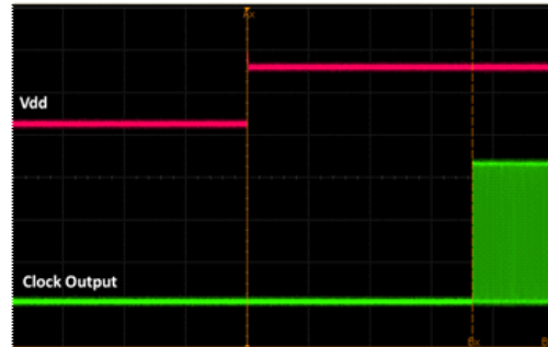
Figure 17. Startup Waveform vs. Vdd
