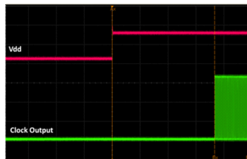
Figure 17. Startup Waveform vs. Vdd
