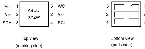
Figure 3. UDFPN5 (DFN5) package connections
