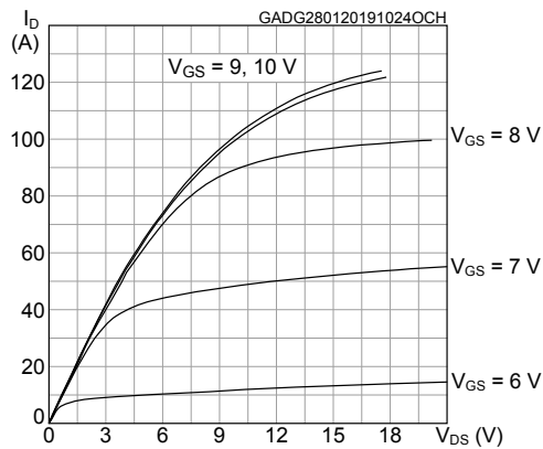
Figure 3. Typical output characteristics
