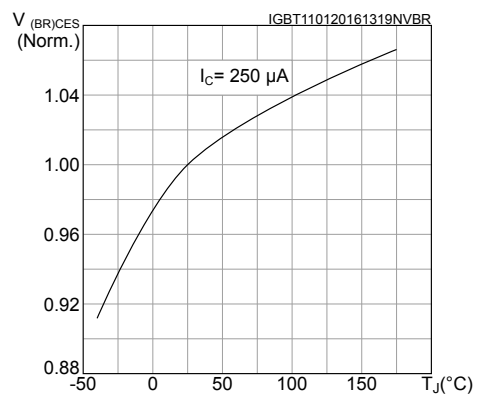
Figure 12. Normalized V_(BR)CES vs. junction temperature
