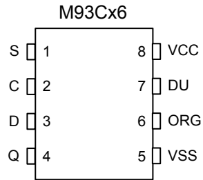
Figure 2. 8-pin package connections (top view)
