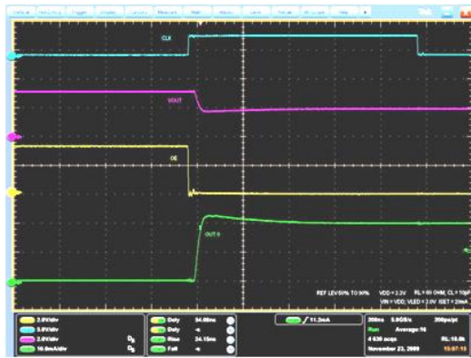
Figure 20: Turn ON output current characteristics (1)
