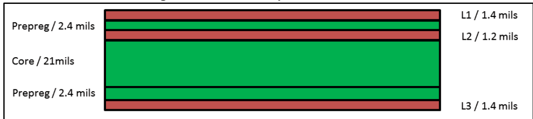
Figure 18: PCB stack-up recommendation
