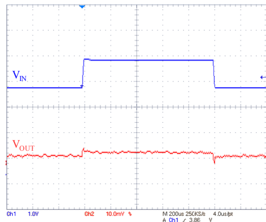
Figure 25. Line transient ( I_{OUT} = 250\text{ mA} )
