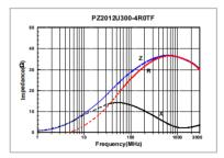
Multilayer Chip Ferrite Bead
