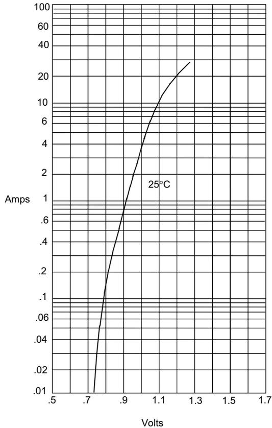
Instantaneous Forward Current - Amperes *versus*
