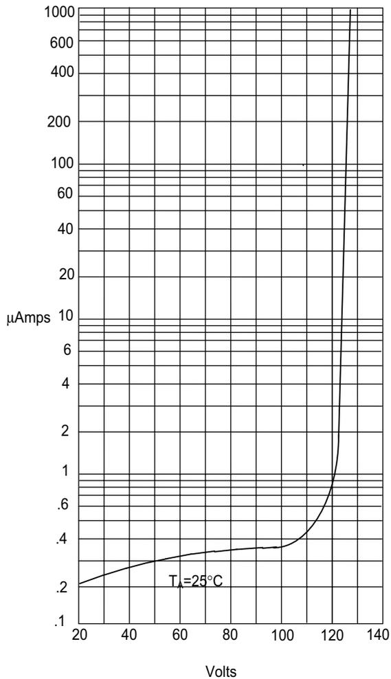
Instantaneous Reverse Leakage Current - MicroAmperes *versus*
