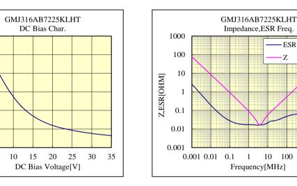
GMJ316AB7225KLHT GMJ316AB7225KLHT Capacitance Temp. Ripple Current 10 100 0 dTemp.[degreeC] dC/C[%] 10 - 10kHz -20 -30 1 -55 -35 -15 5 25 45 65 85 105 125 0 0.5 1 1.5 2 2.5 3 Temperature[degreeC] Ripple Current[Arms]
