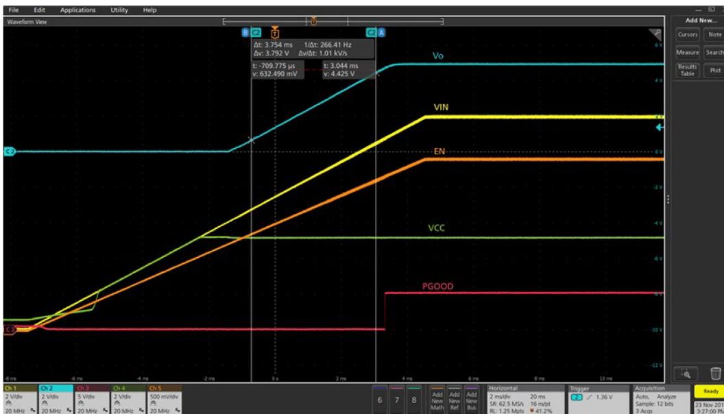
Figure 17 Startup with 3A load (Ch1:PV IN , Ch2: V OUT , Ch3: PGood, Ch4:V CC , Ch5: Enable)
