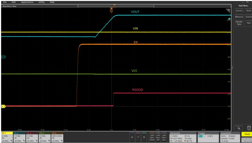
Figure 7 Startup into pre-bias (Ch1:PV IN , Ch2: V OUT , Ch3: PGood, Ch4:V CC , Ch5: Enable)
