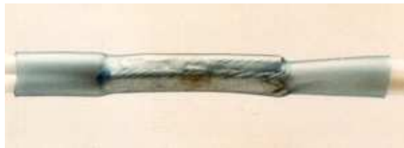
Unacceptable: Insufficient heat. Contour of solder perform is visible.
