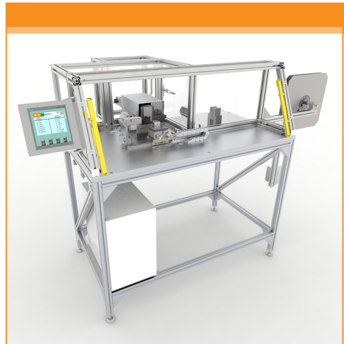
Semi automatic positioning of coil by use of a motor-driven locator unit
