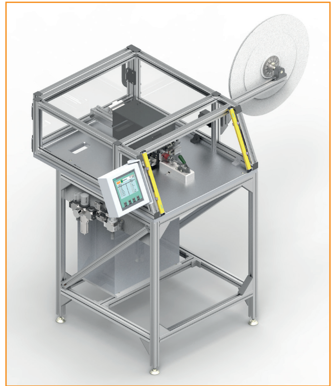
Manual positioning of coil by use of a manually operated locator unit
