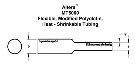
This specification covers the requirements for one type of single wall, electrical insulating, extruded tubing whose diameter will reduce to a predetermined size upon application of heat in excess of 110°C (230°F).
