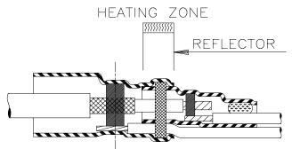
Position the center sealing insert of the SolderSleeve termination assembly whithin the heating tool reflector and apply heat until soldersleeve tubing collapses onto cable dielectric. Move assembly whithin the reflector to the large solder preform and apply heat until it melts and flows forming a solder fillet between the cable shield and the ground wire and then shrink the tubing onto the cable jacket.
